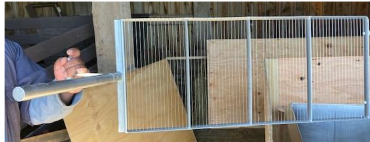
Cheese curd knives (2), needed for cheesemaking. Each harp has a wire missing.
